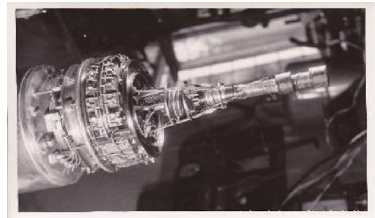
Figure 4: An ultra low part of the cryostat of the dilution refrigerator (approx. 1966).
