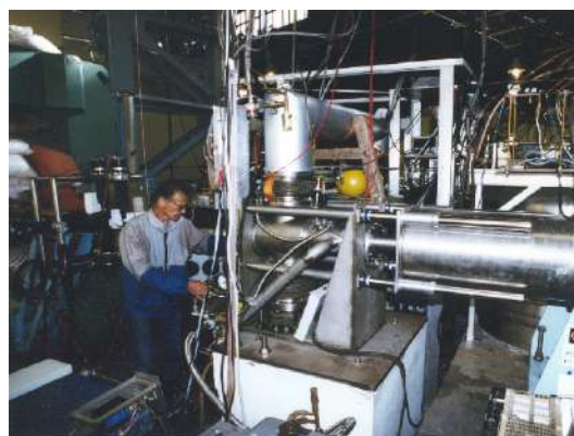
Figure 11: The movable FST for high energy spin physics experiments (Dubna-Nuclotron). This project was supported with INTAS grants in 1993 and 1995.
