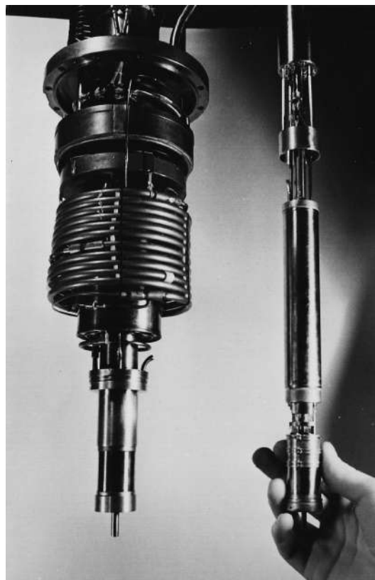
Figure 6: The low temperature unit of the FST and insert for loading target material.
